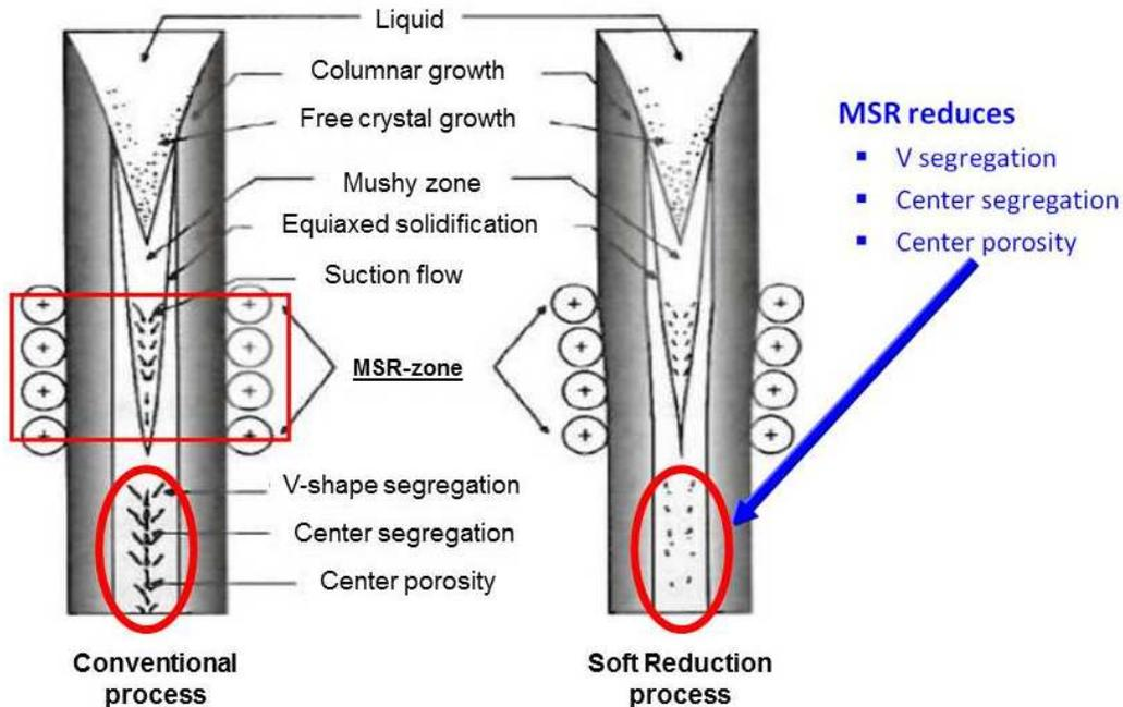
Figure 9. Schematic of continuous casting process without (left) and with (right) mechanical soft reduction. Note box indicating the region on the partially solidified bloom where MSR is applied and ovals noting the improvement in V segregation, center segregation and center porosity that can be achieved with MSR<sup>11</sup>.
