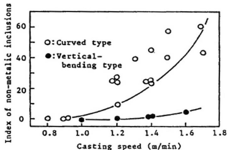
Figure 7. Plot showing the effect of caster design and casting speed on concentration of oxide inclusions.
