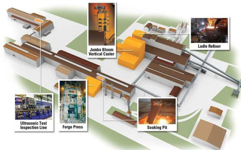
Figure 1. Map of the Faircrest Steel Plant showing the locations of recent strategic capital improvements - jumbo vertical bloom caster (2014), second ladle refining station (2013), inline forge press (2013), ultrasonic inspection line (2012) and additional soaking pit reheat capacity (2011).
