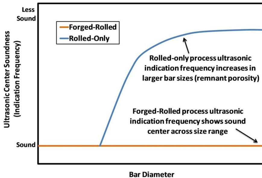
Figure 2. Figure showing the capability of the forged-rolled and rolled-only process. Rolling deformation can leave remnant porosity in larger bar sizes due to the surface-concentrated nature of the deformation. The forged-rolled process is able to fully consolidate the center material and produce large bars which conform to stringent pass/fail soundness specifications.
