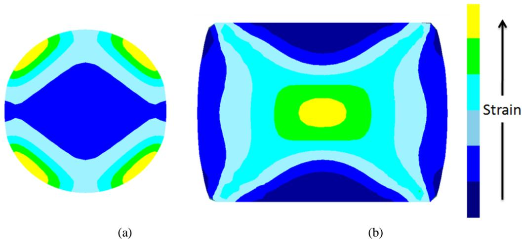
Figure 3. Simulated characteristic strain patterns produced during (a) rolling a quadrilateral to a round and (b) open-die forging. Rolling deformation is localized on the surface, especially near the breakdown of the prior corners, while open-die forging is capable of creating peak strain values at the core.
