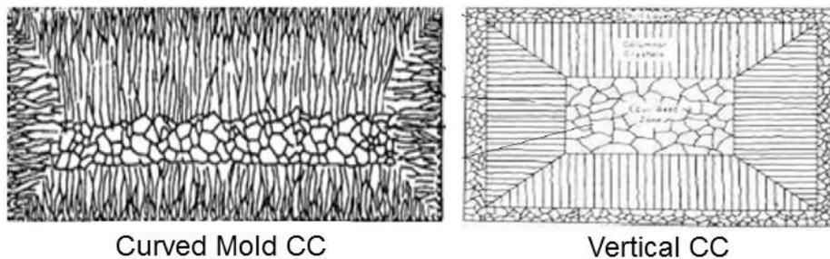
Figure 8. Drawings showing the difference in as-cast structures for curved mold (left) and vertical continuous casters (right).
