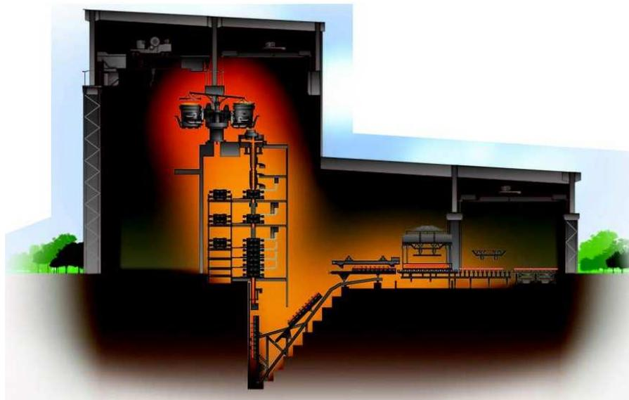
Figure 5. Illustrated side view of the new Faircrest Steel Plant jumbo vertical bloom continuous caster.
