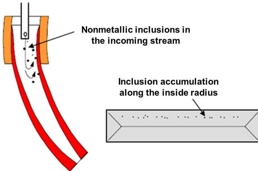
Figure 6. Basis for the formation of an inside radius concentration of oxide inclusions in curved mold casting machines.
